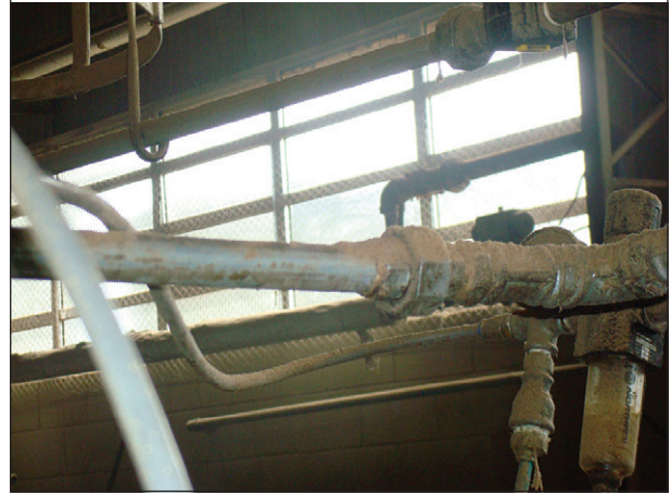
FIGURE 18 Accumulation of product in the equipment, lacking cleaning
